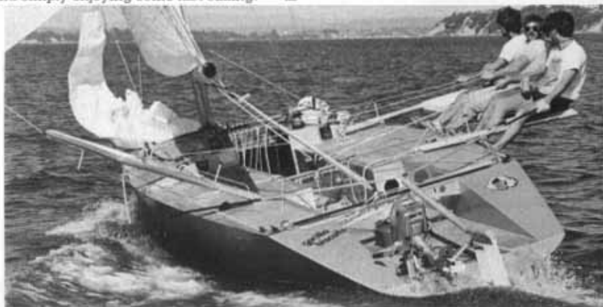
Deck is mostly cockpit, though the crew will spend most of their time on the racks.
