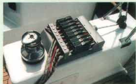
Top: large, well protected cockpit. Above: central power winch with all lines led aft
