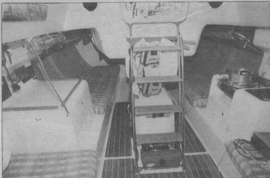
Pipe berths above the quarterberths make up the required number of bunks to conform to the IMS rule.
