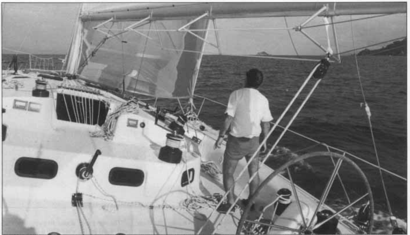
Future Shock's large cockpit extends in "trenches" forward round the cabintop. The single traveller winch is located centrally behind the companionway hatch. The boom, built to be as light as practicable, is a small section with four sets of struts and stays adding stiffness.
